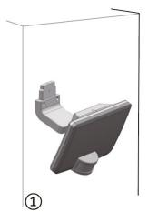
Fix the luminaire to the wall using the screw holes.
